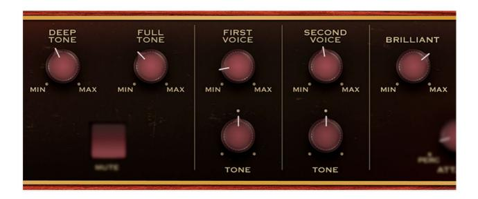
The *Deep Tone*, *Full Tone*, *First Voice*, *Second Voice*, and *Brilliant* knobs each control various filtered versions of the basic Solovox oscillator tone. Unlike typical analog synthesizer filters, the oscillator signal is split and routed to *all* of the filters, processed and then summed together, creating a composite tone, so it's best to think of these knobs as mixer controls. If all of the Tone knobs are set to zero, no sound is heard.
