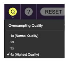
**Q Oversampling Quality -** The Q button sets Solovox's internal oversampling rate; the higher the setting, the better audio fidelity will be, with the caveat that more computer processing power will be required.
